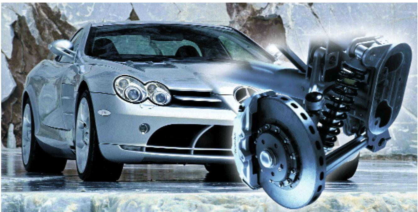
**The Mercedes-Benz SLR uses fiber reinforced ceramic brake discs**
