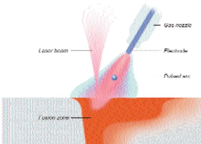
**Schematic representation of laser hybrid welding process**
