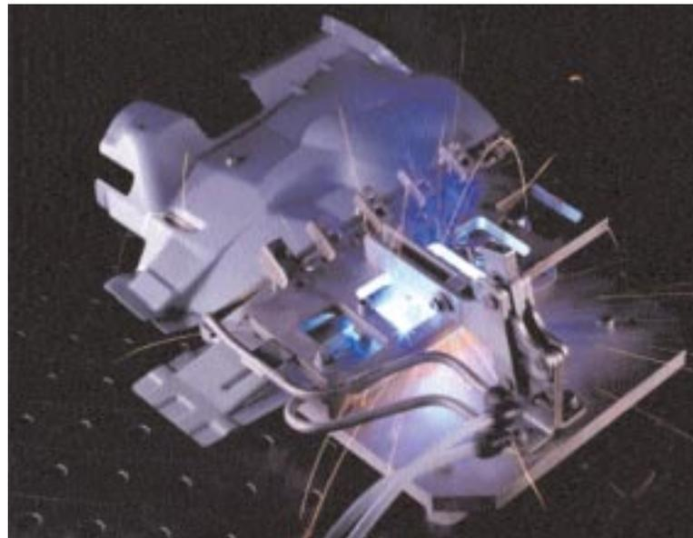
**Trumpf claims that laser scanner welding does not subject parts to wear and tear and exhibits high consistency**
