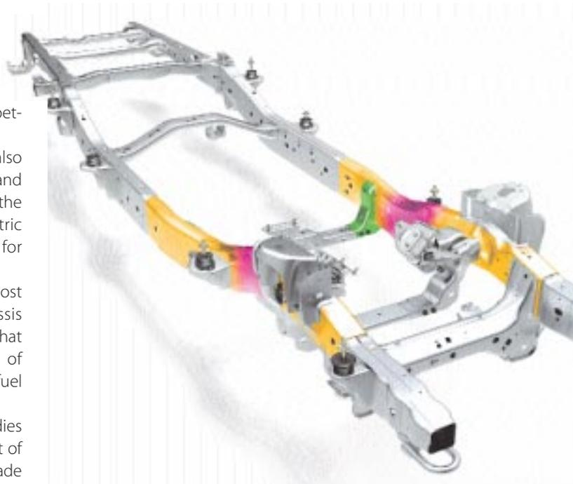
**Dana's use of hydroforming on the Ford F-150 box frame has helped reduce weight**
